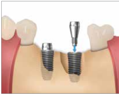
GBR Abutment Connection SuperLine : FX4510SE
